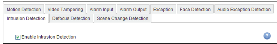
Figure 117, Setting Intrusion Detection on IP Camera
